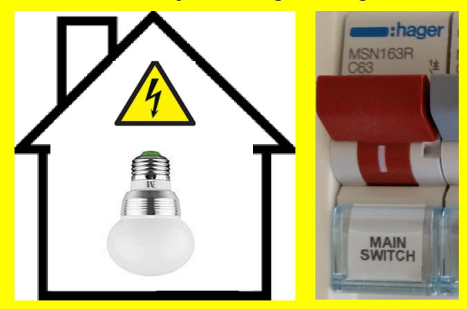
BEFORE YOU CHANGE A LIGHT BULB GO TO THE SWITCH BOARD AND TURN "OFF" THE MAIN SWITCH
