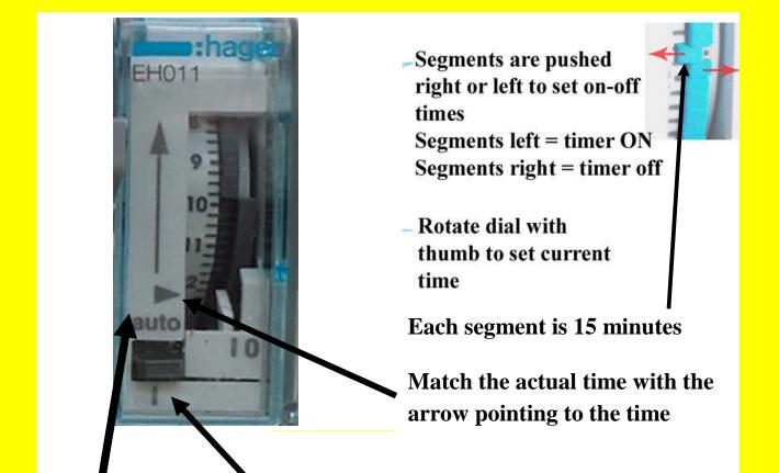
Override timer by selecting the lever indicated to the "I" position by pushing the lever down- *this will allow you to clean the pool or heat more water when the timers is off.*
